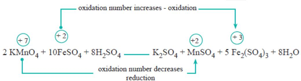
In this reaction, manganese in potassium permanganate (KMnO<sub>4</sub>) favours the oxidation of ferrous sulphate (FeSO<sub>4</sub>) into ferric sulphate (Fe<sub>2</sub>(SO<sub>4</sub>)<sub>3</sub>) by gaining electrons and thereby gets reduced. Such reagents are called oxidising agents or oxidants. Similarly, the reagents which facilitate reduction by releasing electrons and get oxidised are called reducing agents.
